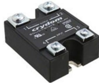
Most electronic switches operate on the “low side” meaning they connect the switched circuit to ground (typically the negative side of the power supply). “High side” switches connect the switched circuit to the positive side power supply and are less common. It is important to select the correct type.
