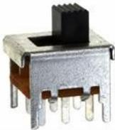
**Slide** – a protrusion is moved to one of several defined positions in a linear arrangement. Two states (on or off) and three (center-off) are common.
