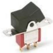
**Rocker** – an actuator (usually concave) is operated by pressing one end or the other. This type typically has two states (one end or the other down) or three (center-off).
